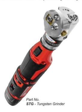
Sharpie grinders deliver quick and consistent electrode grinds for snappy arc starts, better puddle control and improved weld quality. The double-sided diamond wheel easily grinds tungsten electrode sizes, .040", 1/16", 3/32" and 1/8" (1.0mm, 1.6mm, 2.4mm and 3.2mm)
