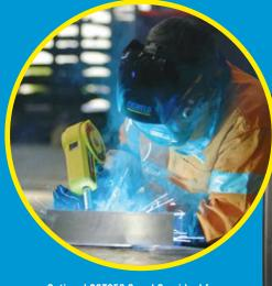
Optional SGT250 Spool Gun ideal for your precision aluminium fabrication, repairs and auto/marine work.
