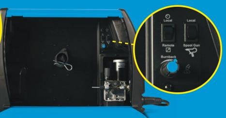
**44 Great feedability and control over my aluminium welds when using the Tweco Spool gun with my Transmig 255i 55**
