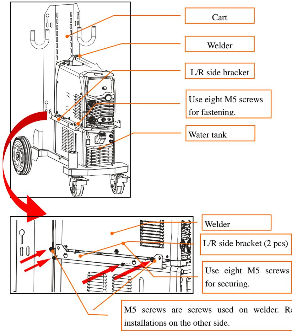
Step 6 Attach support brackets to welder.
