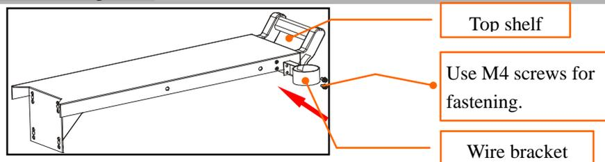
Step 3 Attach water tank brackets to water tank.
