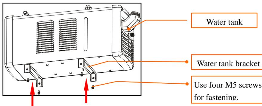
Step 4 Place water tank on bottom base and secure it in place.
