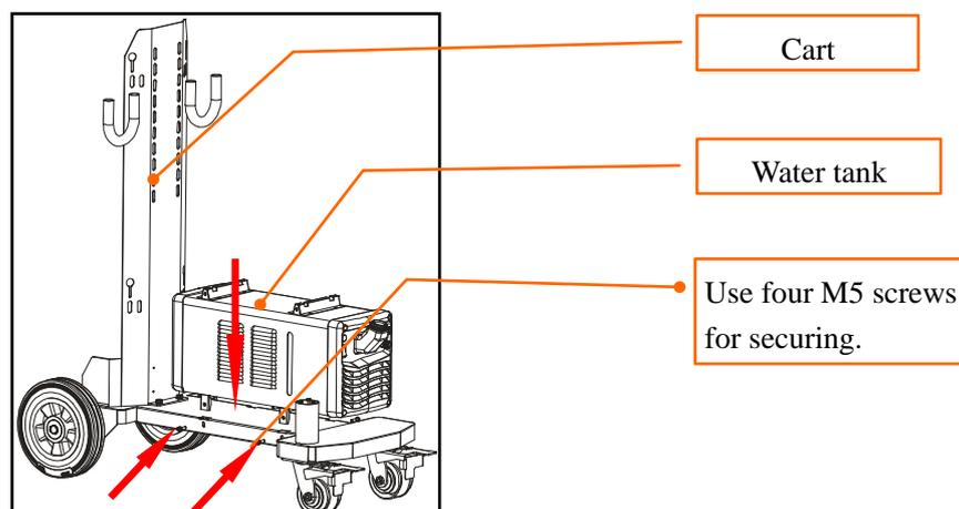
Step 5 Top water tank with welder, have the welder aligned and secured.
