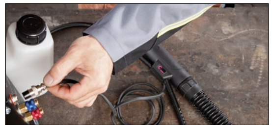
8. Connect the flow control cable to the cooling unit.
