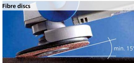
Using COMBICLICK helps to avoid scratches caused by protruding clamping pieces, and exploits the abrasive material that is available.
