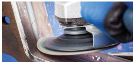
Soft and particularly flexible grinding performance in face-down grinding.
