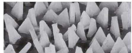
The **VICTOGRAIN** abrasive grain is optimally aligned
