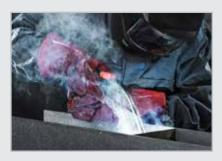
The X3 MIG Welder's MIG/MAG process has been carefully tuned to give the arc outstanding stability, which makes it easy to manage and creates a minimum amount of spatter – also when using inexpensive CO2 shielding gas. When the need for post-weld grinding is reduced, welders can focus on productive weld-ing.
