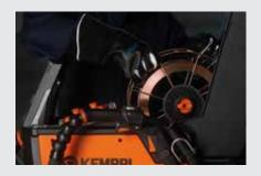
Top-loading wire feeder design ensures ergonomics and safety when changing heavy filler wire spools.
