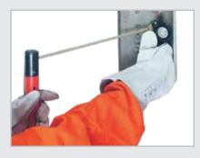
R11-T wireless remote control units can be used simply by touching the electrode
