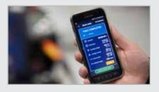
By using the WeldEye mobile application, welders can browse their company's WPS library, receive digital work orders, report work progress, and get feedback on their welds – including heat input values.
