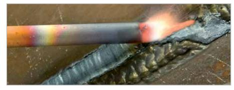
KempGouge ARC 800 makes easy work of carbon arc gouging tasks.
