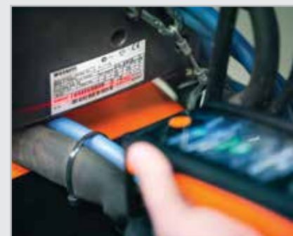
ArcValidator RC records all individual validation process data for later transfer to the PC software.
