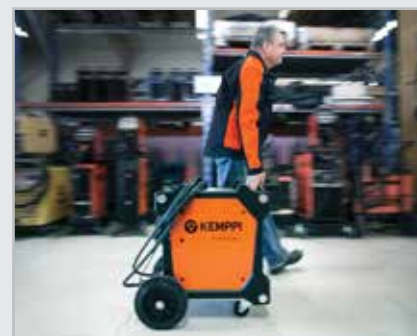
ArcValidator load bank is easy to move around and a universal solution for multi-branded fleet validation.
