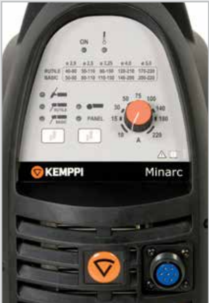
Minarc 220 is easy to set. Electrode type selection ensures the best welding quality and you can also use an optional remote control to make fine current adjustments during welding.
